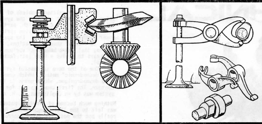
The Bigean-Sport desmodromic system was unique with its rotating swash plate and cross-head with rollers.
