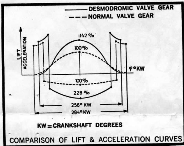
With a desmodromic system the rates of opening and closing the valves may be fiercer with no danger of valve float.
