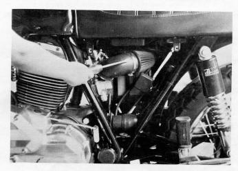
I took the back light wiring out from under the fender, taped it up real neat, and left it exposed on top of the fender. Big bumps when two-up caused the tire to expose several spots in the wiring harness.
