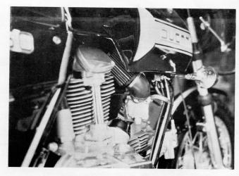
Note how filters tuck away neatly away from rain blast. Above photo: Note the modification to side cover to expose view to rear cylinder.
