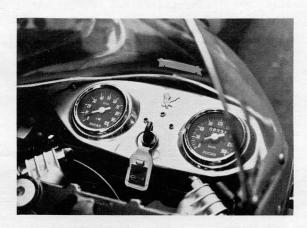
The instrument panel is machined aluminum from stock aluminum block, instruments are Veglia instead of that cheap Smith crap, the eagle at the center of the panel is 18K gold. A small portion of the Bimota Clip-ons are visible in this photo.
